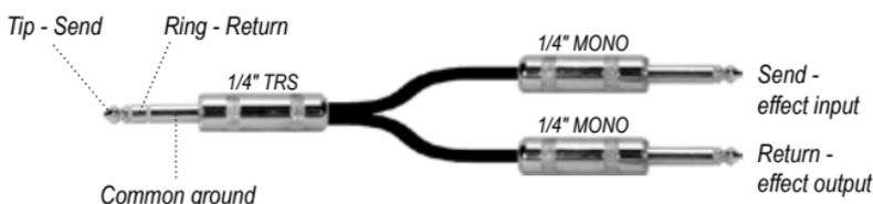
The TRS plug connects to the Bassbone LOOP jack and the two 1/4" mono plugs connect to the input and output jacks of the effect pedal.
