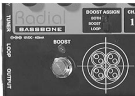
Being able to engage both the boost and the effects loop with a 'single foot action' adds tremendous flexibility while reducing 'tap dancing' on stage. For instance you may want to kick the bass up a notch and introduce a flanger at the same time. For this, the BOOST ASSIGN switch would be set to BOTH. This has the advantage of keeping noisy effect devices out of the signal chain when not being used.
