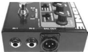
It is important to note that unlike a direct box that would normally be connected before the Bassbone, the XLR out is post Bassbone. This means that all of the Bassbone EQ and volume settings will be heard on the XLR output. This is particularly advantageous when playing gigs without a sound
