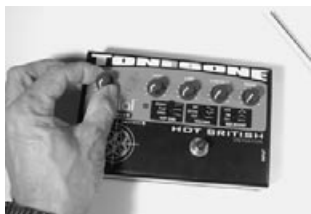
Press on knobs with shafts counter-clockwise and pointers at 7 o'clock.
