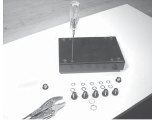
Knobs off, nuts & washers off, side jack nuts & washers off, now remove screws.
