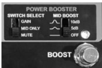
There are also two slider switches that are associated with the boost circuit. The first switch assigns the way the foot switch is being used. There are 3 settings:
