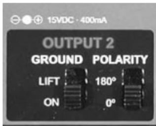
Now listen to the residual noise. Try lifting the ground switch on output 2(B). If you cannot hear a difference, then leave the ground connected. Now try reversing the polarity. This will give you a sense of spaciousness when *out of phase* and a more unified and centered sound when *in phase*.
