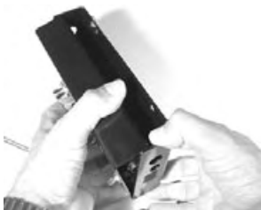
Spread chassis sides to clear input & output jacks.
